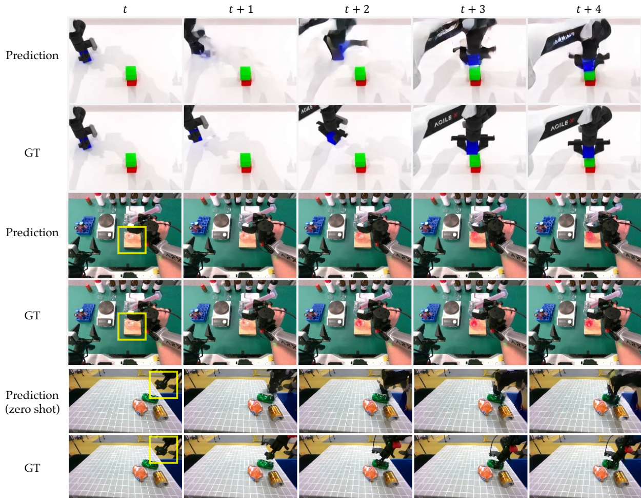
Figure 11. Foresight-conditioned future rollouts from the frozen world model. The model predicts future frames ( t \sim t + 4 ) conditioned on foresight embeddings extracted from the VLM context, demonstrating both accurate motion prediction and physically consistent scene evolution.
